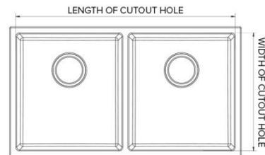
3. Drill holes for the fasteners on the underside of the countertop surface. Holes should be drilled at an even distance from one another and around 1" from the cut-out edge. Attach the mounting clips.
