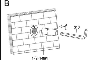
**2.** Fix the faucet body to the reserved water pipe with 1/2-14NPT thread in the wall.
