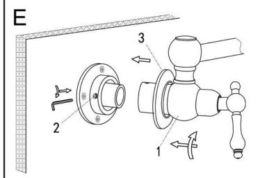
**5**. The decorative cover needs to be close to the wall, and the outlet is straight down after correct installation like the above figure.
